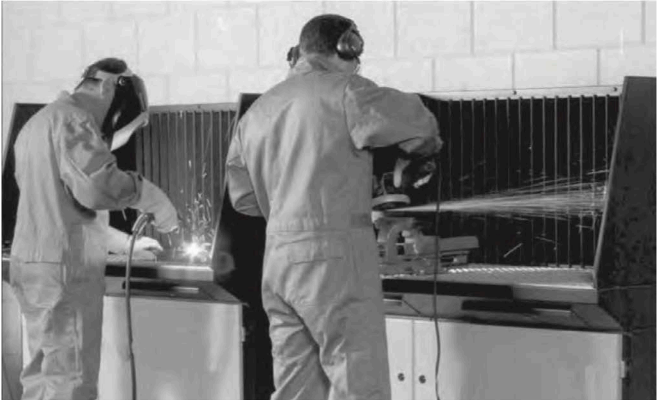
Figure 2: Source capture method – downdraft welding bench. Courtesy Plymovent North America
